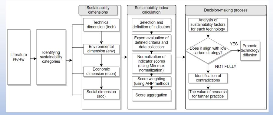
The core element for sustainability assessment is the construction of the composite sustainability index. In this study composite sustainability index is calculated for district heating (based on the natural gas) and four different technological solutions of decentralized (individual) heating wood pellet boiler; natural gas boiler; solar collectors; and (4); heat pump.
