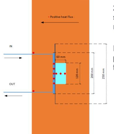
2D model of the test stand with the PCM sample in the center and Hot/Cold plate right next to it.
