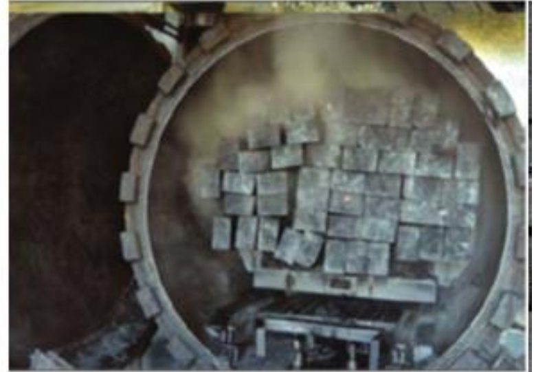
Figure 3. View of autoclave for impregnation with the Rüping method ( Wojciechowski et al 2018 )
